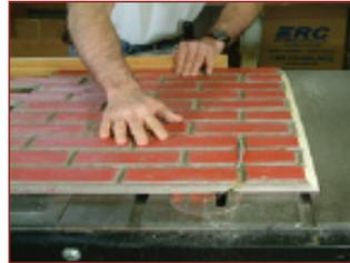
2. Cut the panel at a 45 degree angle. TIP: A simple panel cutting jig helps to do this on a table saw.
