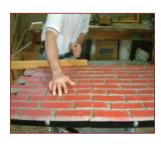
3. Take the leftover panel and flip it around 180 degrees. You will be cutting a 45 degree angle reversed to the last cut.
